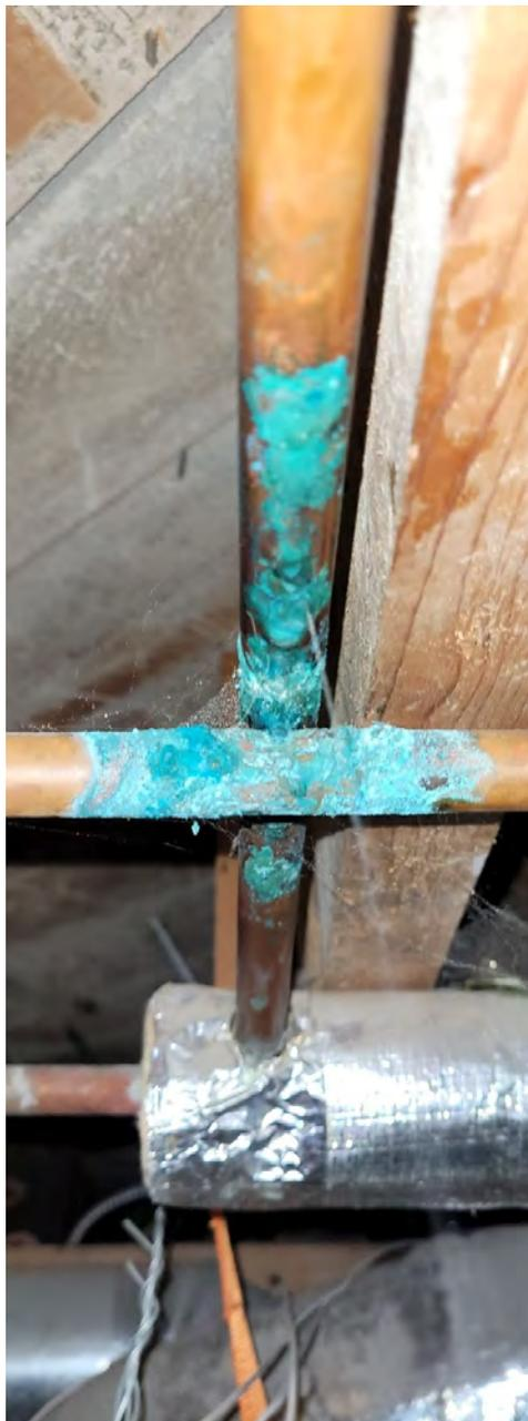
This week we had a leak at my house. It wasn't a bad one, just a corroded pipe that I noticed when I walked into the laundry room and felt it drip on my head. I tried to fix it myself, it started dripping faster, and so I called my landlord and she in turn got a plumber to come in and fix it. In the meantime though, my pipe was still leaking, so we turned to that oldest of drippy-pipe solutions: the bucket.
